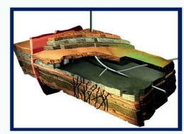
A reservoir section illustrating a standard well to multilateral well
